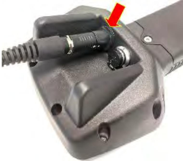
Fig 3. Cygnus 1 Ex Probe Connector.
