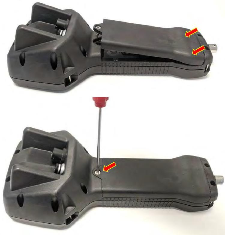
Fig 2. Cygnus 1 Ex Battery Pack Fitting.
